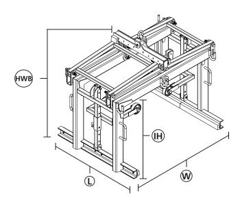
Designed and manufactured to lift palletised blocks and bricks. The CA105AE Block Grab is also suitable for handling all types of concrete products such as slabs, steel strapped bricks, blocks, kerb stones and paving blocks.
